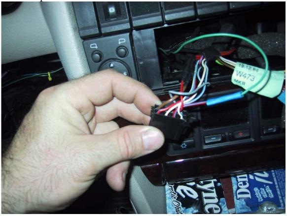
Route the new wire to the K line. In simple terms, the K line is what VAG-COM uses to talk to the car. You will need this because your Concert needs to know if your car has BOSE. You can also use VAG-COM for radio diagnostics, if needed. Anyway, route the wire under the steering column and up the relay board under the hood. Attach the wire to the K terminal (the one with all the green/block string wires going to it)
